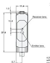
Metal case type 23.4 Two, M3 22 39.3 25.4 4.25 dia. vinyl-insulated round cable with 4conductors (Conductor cross section:0.2 mm² (AWG24), Insulator diameter: 1.1 mm), Standard length: 2 m
