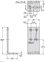
**Photoelectric Sensor Accessory** are installed (Example of E3AS-F1500□)
